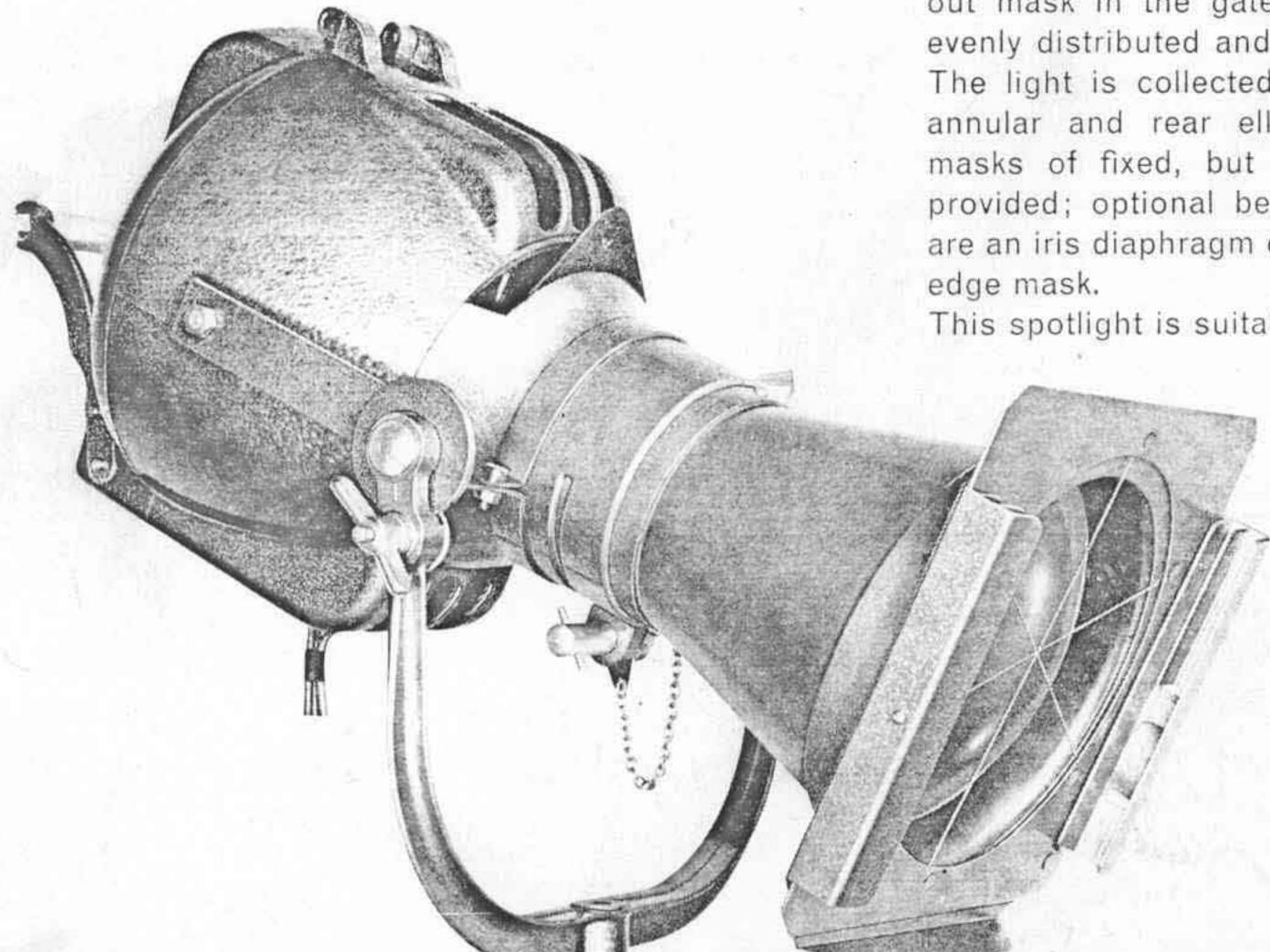
This spotlight projects a high intensity narrow angle beam of any profile determined by a cutout mask in the gate runners. The beam is evenly distributed and has clear cut edges. The light is collected at the gate by a front annular and rear ellipsoidal reflector. Four
